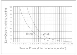
Performance curve results using a  $1\!\!/_3$  and  $1\!\!/_2$  HP pump with (2) fully charged Power+ 100 amp hour batteries.
